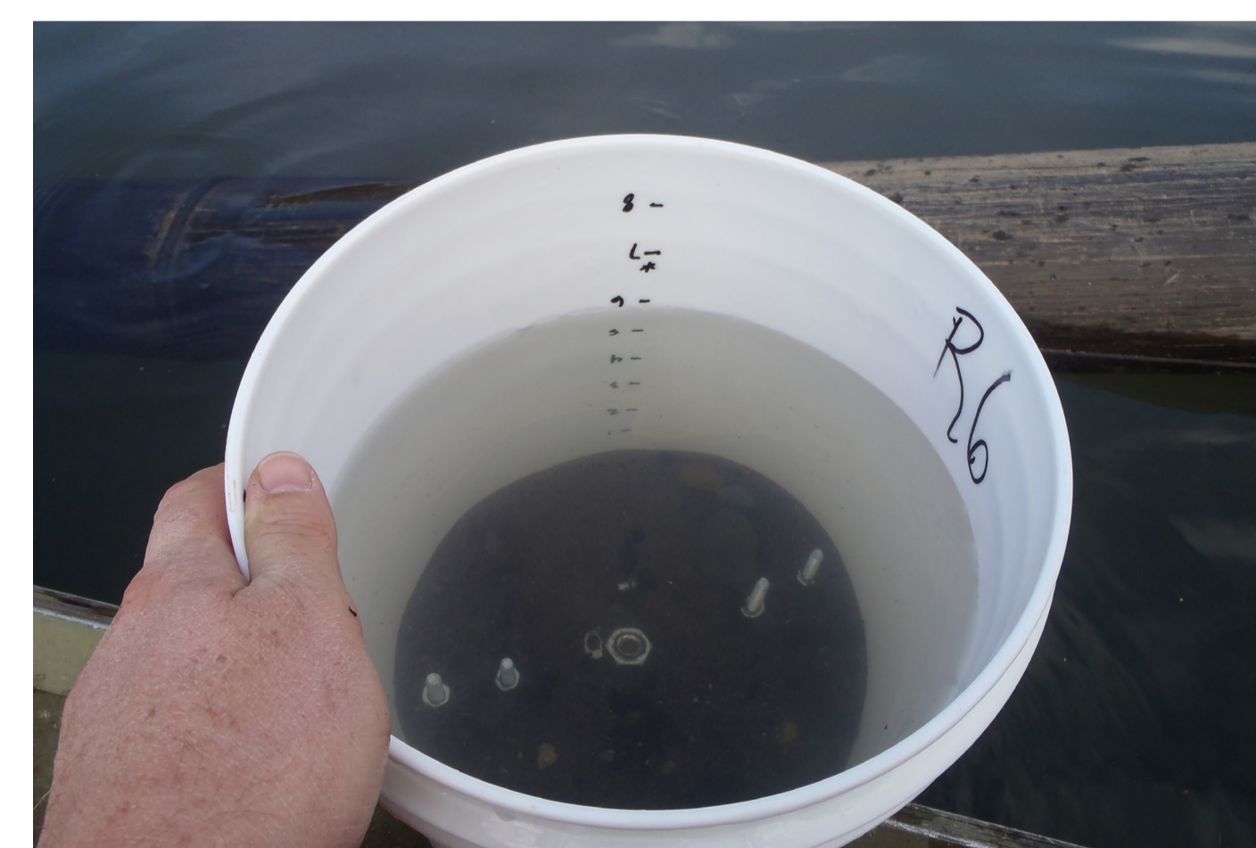
Cap thickness confirmation by rain gauge method
